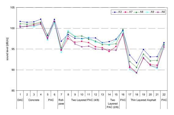
Figure 5: CPX rolling noise levels for all A-candidate tyres on different surfaces
