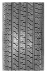
Figure 7: The chosen replacement for tyre A; i.e. the ASTM SRTT tyre
