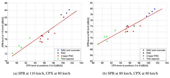
Figure 4: Correlation between passenger car SPB levels and average CPX levels using Tyre A6
