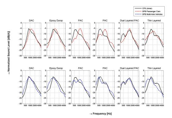
Figure 6: Comparison of SPB spectra and normalised CPX spectra measured using tyre A6 ("inner" microphone positions; i.e. 1 and 2 or 3 and 4 only)
