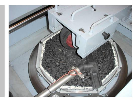
Simulation of tyre and surface wear with "rotating surface abrasion test"
