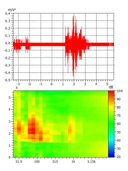
Figure 5. Example of a multi channel synchronised vibration and sound analysis, with multiple analysis options. A vibration signal as function of time (top) and the Campbell diagram of a sound measurement. Both during the passage of a truck.
