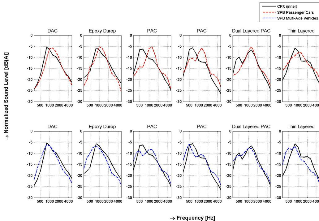
**Figure 6:** Comparison of SPB spectra and normalised CPX spectra measured using tyre A6 ("inner" microphone positions; i.e. 1 and 2 or 3 and 4 only)
