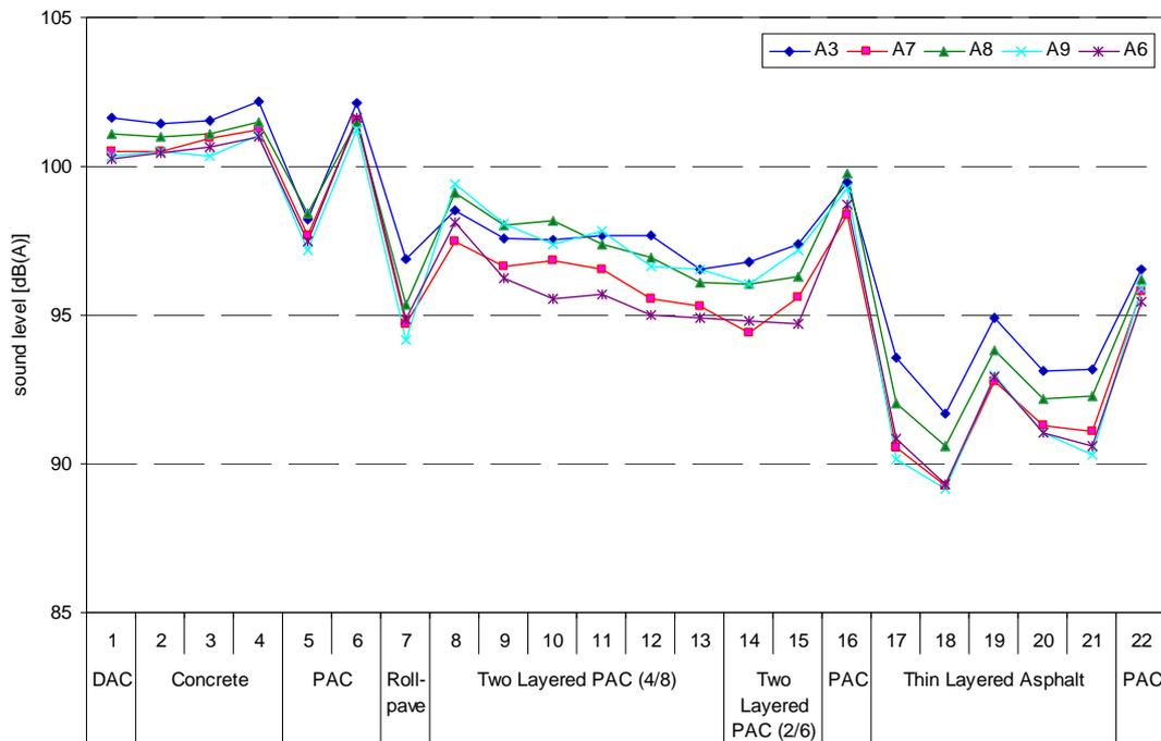
**Figure 5:** CPX rolling noise levels for all A-candidate tyres on different surfaces
