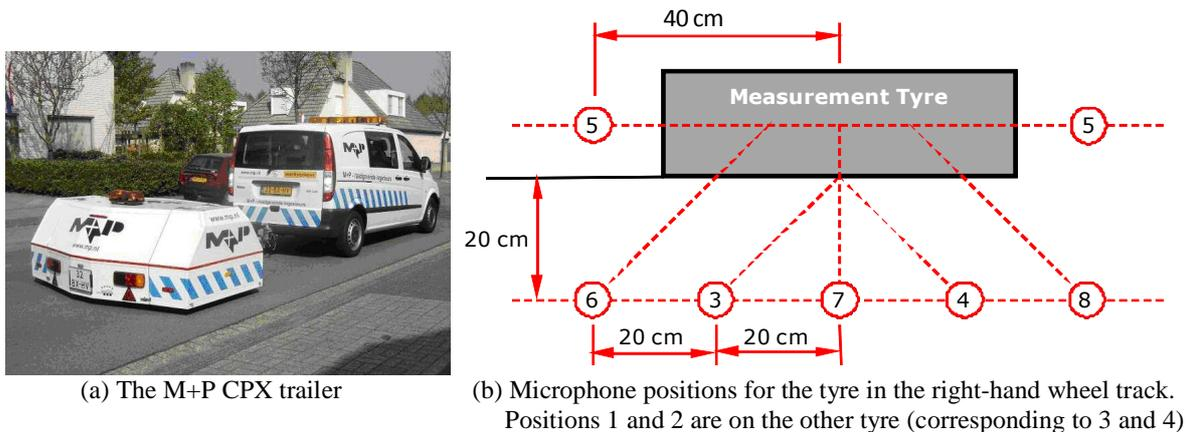
**Figure 1:** CPX trailer and microphone positions used in the study
